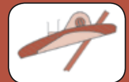
Integral disc ring and bushings on sizes 10" and smaller
