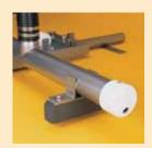
The suction header glides over the surface, removing sludge without causing disturbance, maintaining sludge quality.
