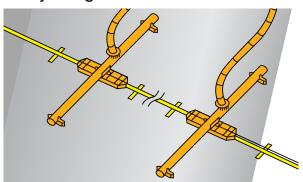
The CT2 sludge collection system can be designed to compensate for high-solids-production water with a double header driven by a single cable system. The travel length of the header is designed to draw the desired amount of sludge from the basin where sludge production is greatest. Double headers also accommodate extra-long basin design.
