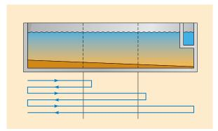
Leopold controls for the CT2 sludge collection system can give each plant the flexibility to meet its individual needs. For example, in sedimentation basins sludge settles unevenly, with more accumulating in the inlet area than in other areas of the basin. Advanced Leopold controls can be programmed to increase sludge removal at the inlet of the tank to even out the sludge load, providing consistent sludge for thickening and disposal.
